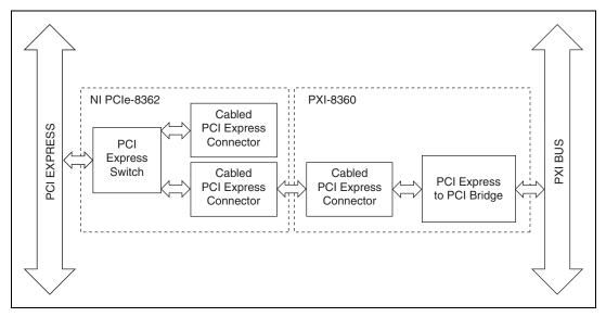
Figure 3-1. MXI-Express Block Diagram with NI PCle-8362
